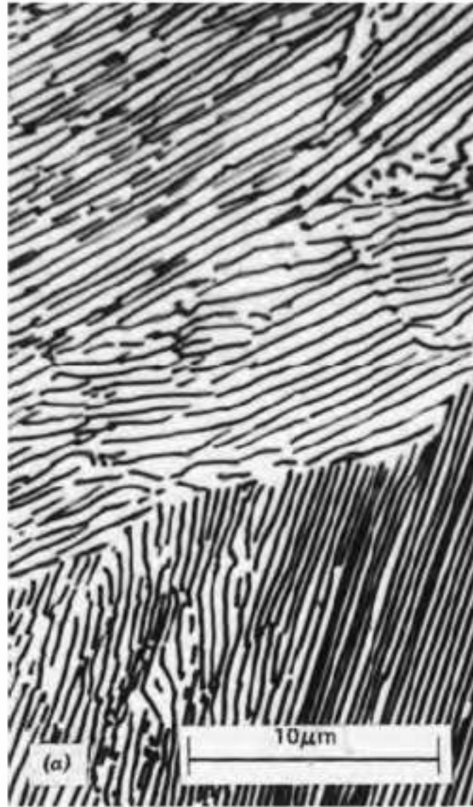
Figure 10.15 Photomicrographs of (a) coarse pearlite and (b) fine pearlite. 3000 \times . (From K. M. Ralls et al., An Introduction to Materials Science and Engineering , p. 361. Copyright \copyright 1976 by John Wiley & Sons, New York. Reprinted by permission of John Wiley & Sons, Inc.)
