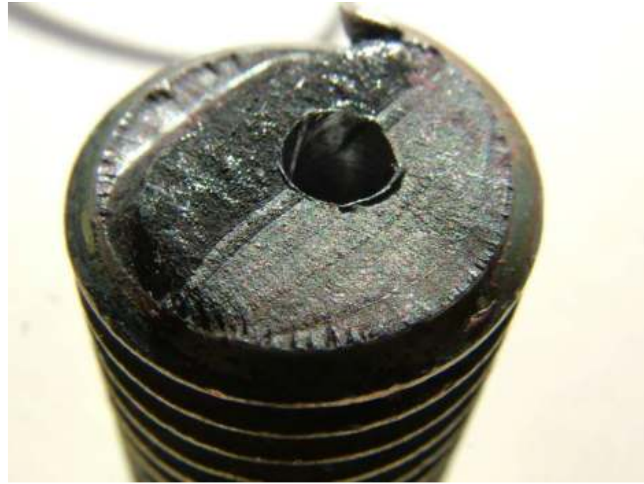
Figure 8.21 Fracture surface of a rotating steel shaft that experienced fatigue failure. Beachmark ridges are visible in the photograph. (Reproduced with permission from D. J. Wulpi, Understanding How Components Fail , American Society for Metals, Materials Park, OH, 1985.)
