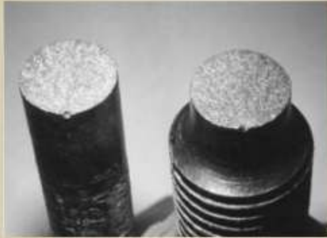
Brittle fracture in a mild steel
