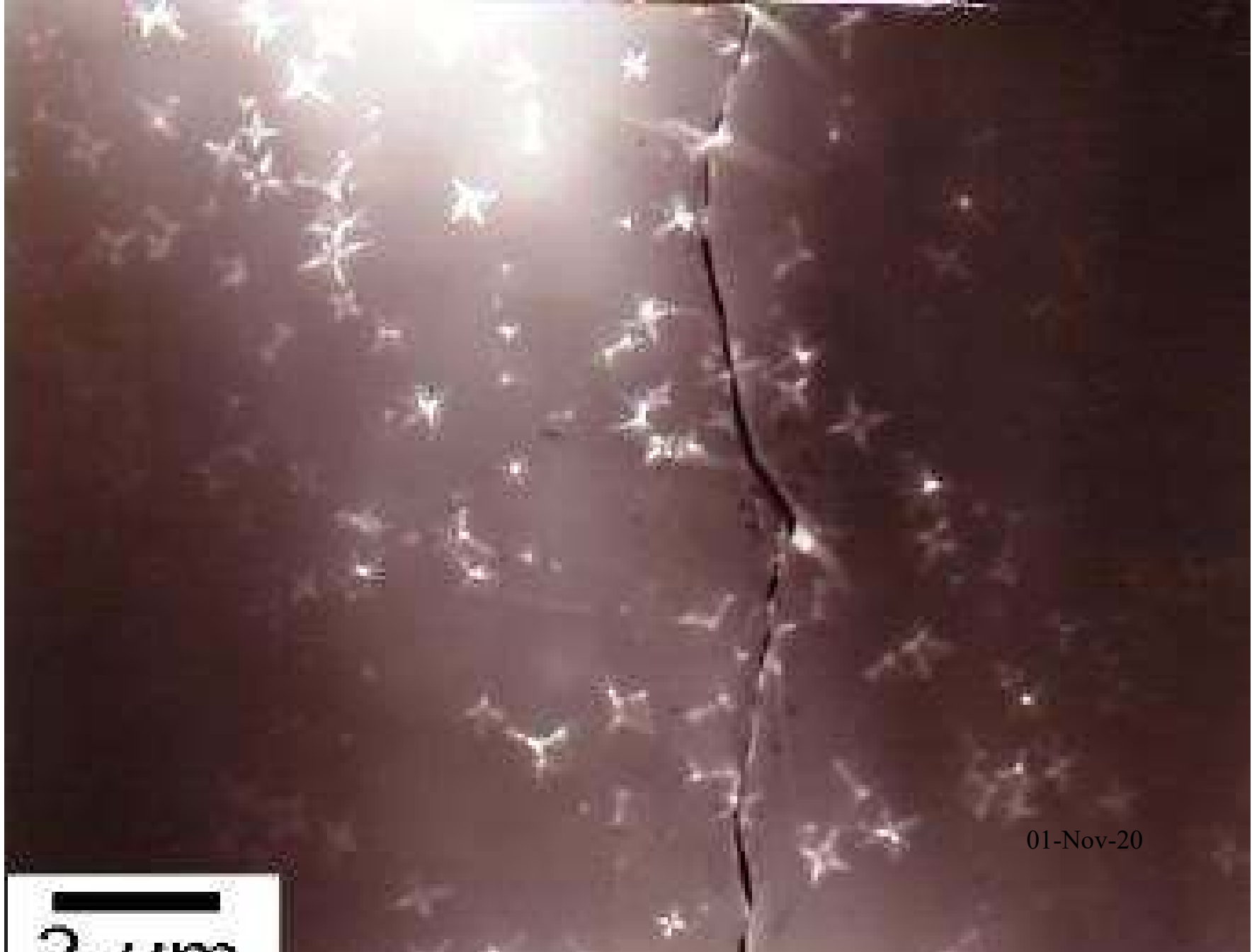
Dendrites forming in Fe 82 Si 4 B 14 metallic glass.
