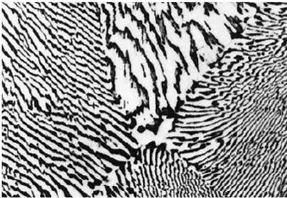
Figure 9.14 Photomicrograph showing the microstructure of a lead-tin alloy of eutectic composition. This microstructure consists of alternating layers of a lead-rich \alpha -phase solid solution (dark layers), and a tin-rich \beta -phase solid solution (light layers). 375 \times . (Reproduced with permission from Metals Handbook , 9th edition, Vol. 9, Metallography and Microstructures , American Society for Metals, Materials Park, OH, 1985.)
