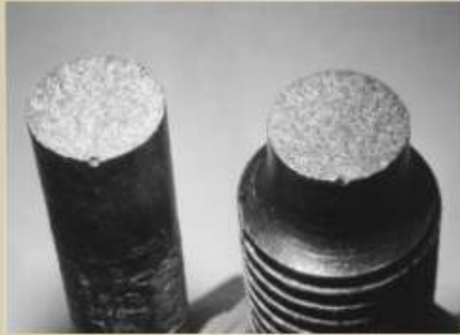
Brittle fracture in a mild steel
